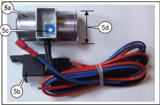
Before you begin, ensure that the Revotec controller tube size (5d) is correct for your radiator hose. Note: The direction of coolant flow through the controller is not important. Failure to use the controller with the relay included will void the warranty.
